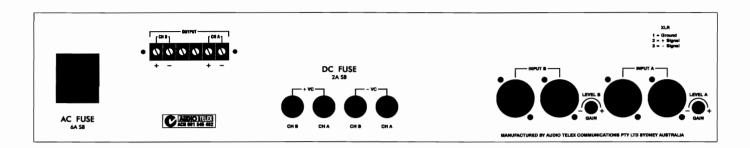
3 Pin IEC, AC Mains Power Inlet: The operating voltage is 240 VAC @ 50 Hz or 110 VAC @ 60 Hz. The AC power voltage level is **not** externally user selectable but is factory pre-set (via transformer selection). The inlet is equipped with an inbuilt AC fuse holder fitted with a 6 Amp slow blow fuse plus one spare fuse. Power consumption is 400 VA. Please ensure that the mains power cord is disconnected before attempting to check or replace this fuse.
