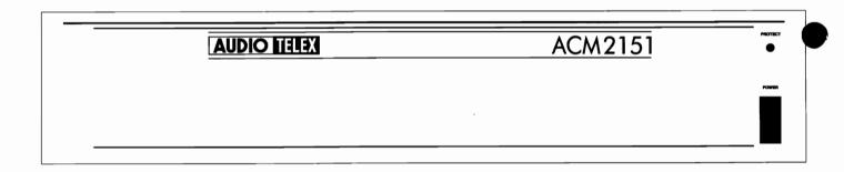
**Power Switch:** The rocker switch located on the front panel turns AC power on to the ACM2151. When the AC power is 'on', the neon in the power switch will illuminate.
