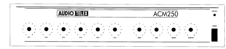
**Dual Microphone/Line Gain Controls:** The 6 dual mic/line input controls are labelled Ch 1 through to Ch 6 and should be adjusted to provide the required level mix for each individual channel. Start with the controls set to level 0 and turn the controls clockwise until the desired mix level for each channel is reached.
