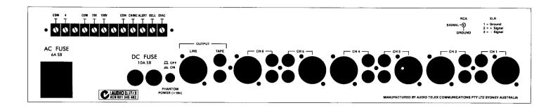
**3 Pin IEC Mains Power Inlet:** The operating voltage is 240 VAC @ 50 Hz or 110 VAC @ 60 Hz. The AC power voltage is factory set and not externally user adjustable. The inlet is equipped with an inbuilt AC fuse holder fitted with a 6 amp fuse plus a spare within the holder. Power consumption is 400 watts.
