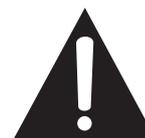
The exclamation point within an equilateral triangle is intended to alert the user to the presence of important operating and maintenance (servicing) instructions in the literature accompanying the appliance.
