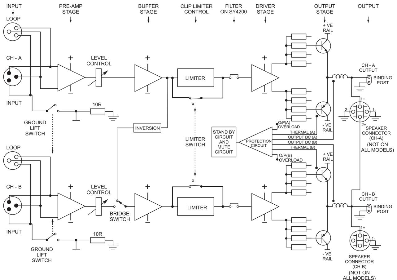
Figure 1 Amplifier Block Diagram
