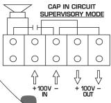
Move RED wire located on the side of the transformers tapping block to the required tapping position.
