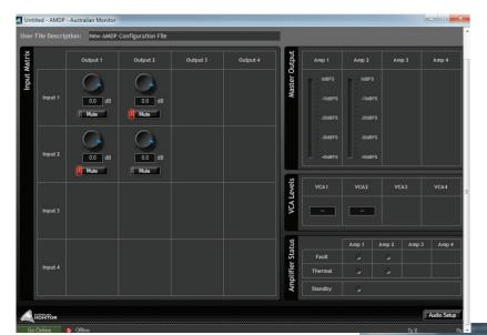
Opening software page allowing input cross mix level, channel input mix mute, VCA values, amplifier fault conditions and LED output level meters in dBFS
