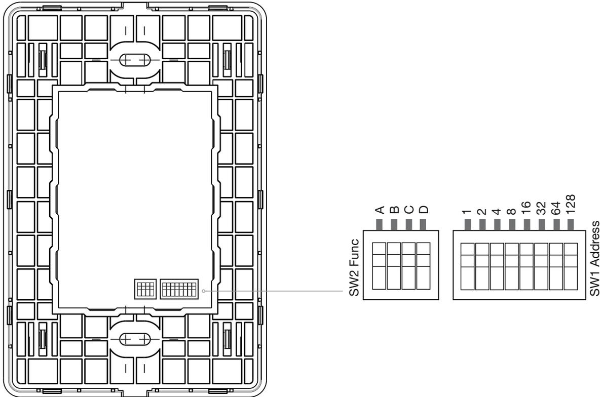
The Revolution series control panels (ICON-CP) have two banks of DIP switches on the rear of the control panel. The first bank of switches labeled SW1 allows the user to address the panel for RS485 communications. The second bank of switches allows the user to set up the LED functions for the remote panel.
