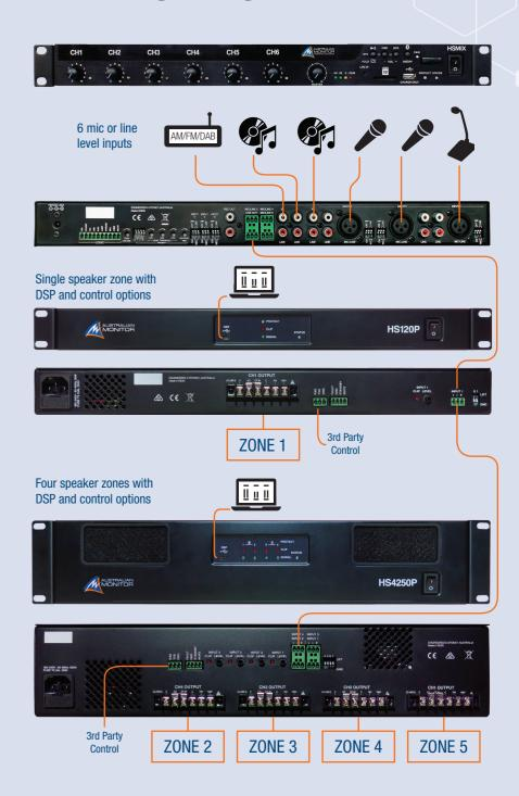
Mini DSP includes - Volume controls, input / output routing, high and low pass filtering, compressor / limiter, pink noise / sine wave generator, muting and inversion.
